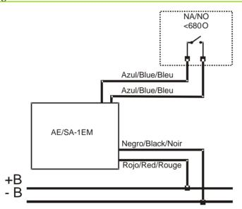
The AE/SA-1EM module must be installed inside the equipment whose signal must be controlled, or in a box arranged for this purpose.
